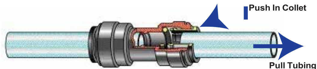
How to Use Quick Connect Fittings
