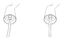
Pass the other end of the tube through the support base and hook the base itself to the Tower.
