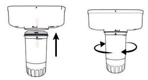
In case of connection of the DDL4 base to a further device, keep the blue clip holder on the rear fitting, push the fitting ring and pull off the cap.
