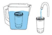
Plug the filter from bottom to top by aligning both arrows, then turn clockwise to align the bar. To remove the filter, turn it counterclockwise and keep it downwards.
